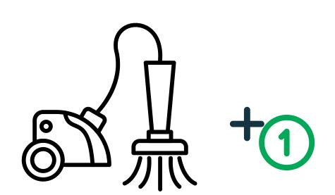
Level 3: Use on tool dust extraction and one other silica control measure
