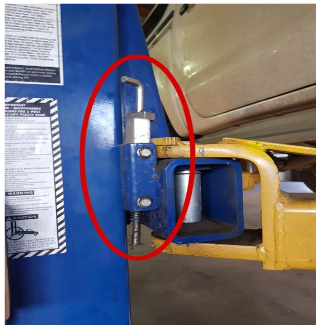
Image 6: Locking mechanism overridden. Locking mechanism is disengaged and rotated out.
