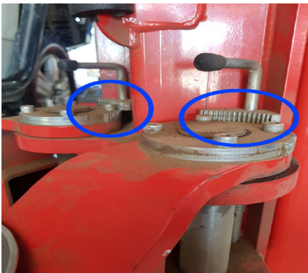
Image 1: Both locking mechanisms disengaged as gears overlap. Vehicle hoist arm can move if force is exerted on the vehicle.
