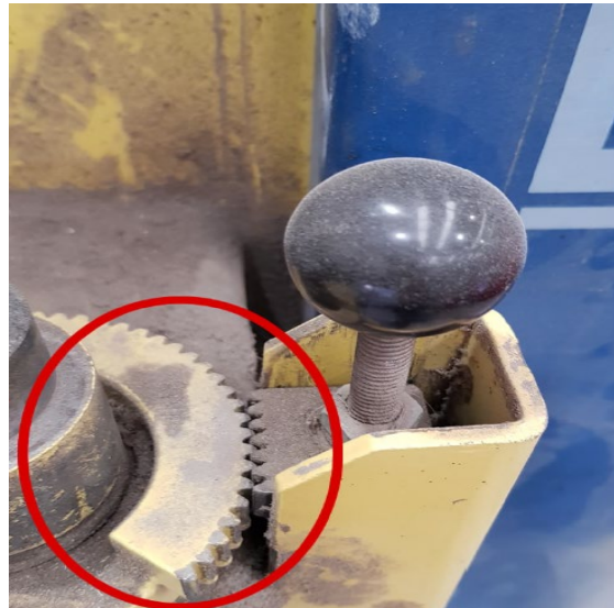
Image 8: Locking mechanism on one swing arm. Locking Mechanism engaged as gears align. Vehicle hoist swing arm cannot move.
