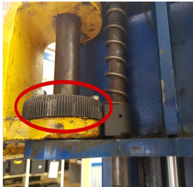
Image 4: Gear teeth are broken
