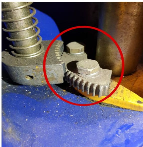
Image 5: Internal locking mechanisms partly engaged.
