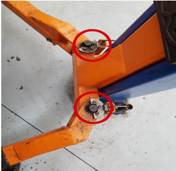
Image 7: Top view of locking mechanisms on hoist arms – two locking mechanisms on one side of the vehicle hoist.
