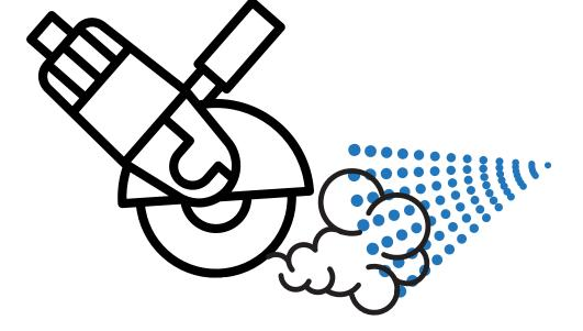
Suppress the dust using water or another wet method
